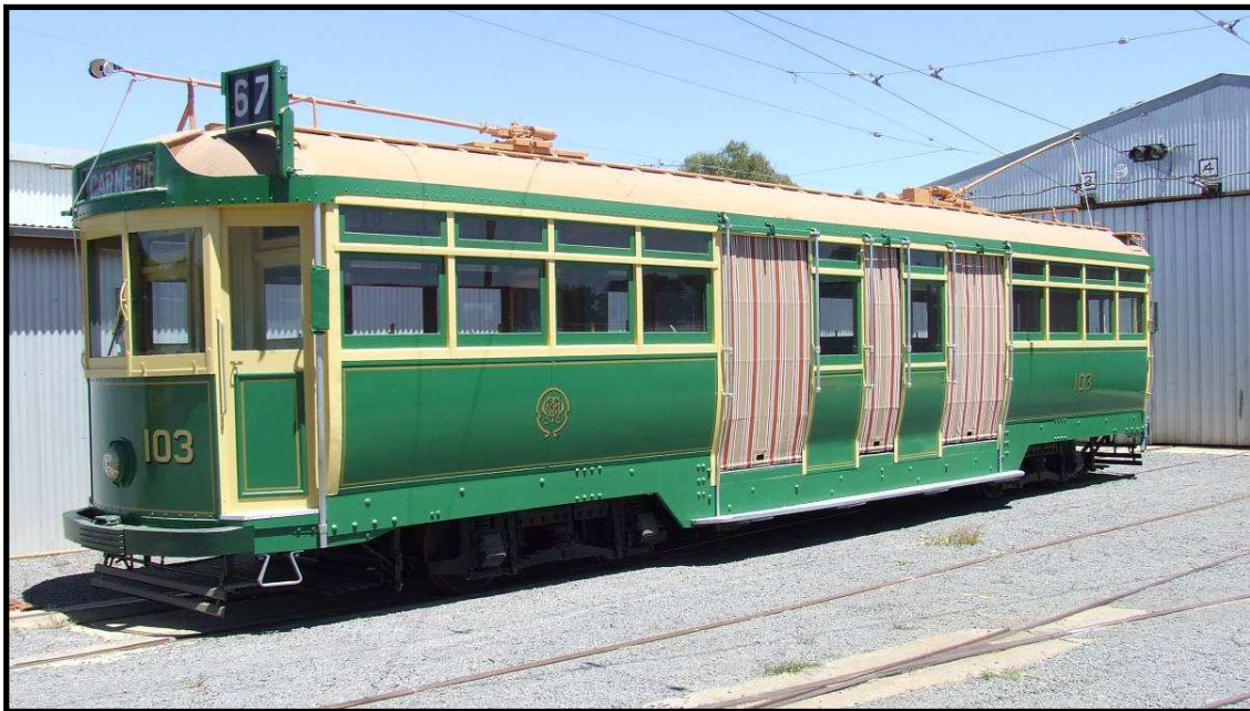
L 103 proudly shows off its new weather blinds. The set in W4 670 have the same colour and pattern. Photo – Anthony Smith.
