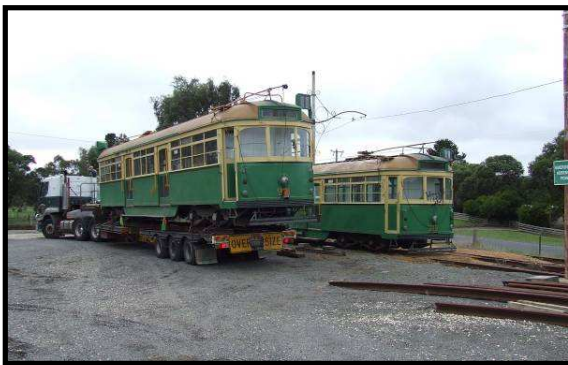
SW6 919 and 931 at the Lower Terminus. Although at first glance they seem ok, both have severe structural faults and are missing many components. Photo – Anthony Smith.
