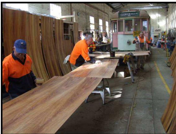
The Bendigo Tramways coachbuilders preparing the plywood sheets for the roof of W3 663. Photo – Anthony Smith.
